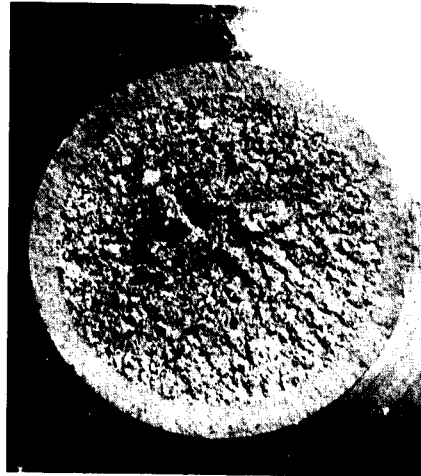
Fig. 28 Fracture surface of prenotched steel bar showing annular fatigue crack
