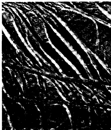
Fig. 4 Rimmed 1008 steel with Lüders bands on the surface as a result of stretching the sheet just beyond the yield point during forming
