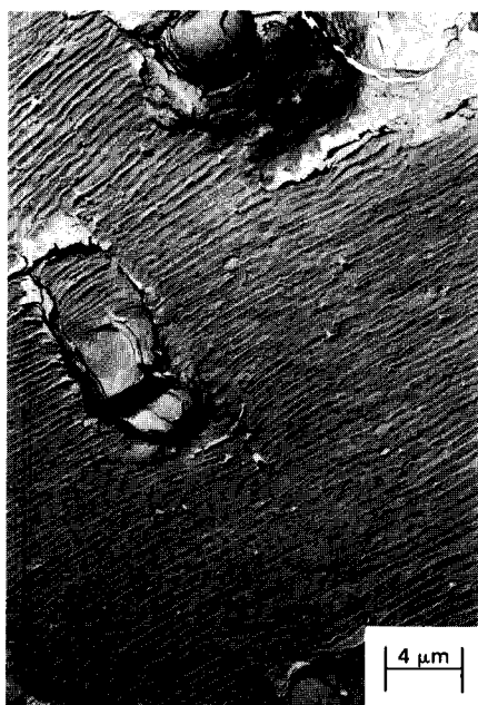
Fig. 17 Transmission electron fractograph (replica) of ductile fatigue striations in 2024-T3 aluminum
