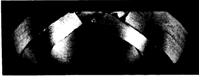
Fig. 6 Shear cracks in a 72% compressed specimen of AISI-SAE 4340 steel
